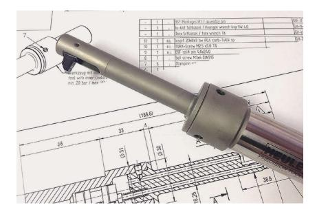
Sicom Industries needed a way to automate the process of moving a tool through a bore without removing and reattaching the cutting head. Coolant pressure is used to retract the cutting blade on Heule's back spotfacer (BSF), independent of spindle direction or contact mechanism. This made retraction reliable.
